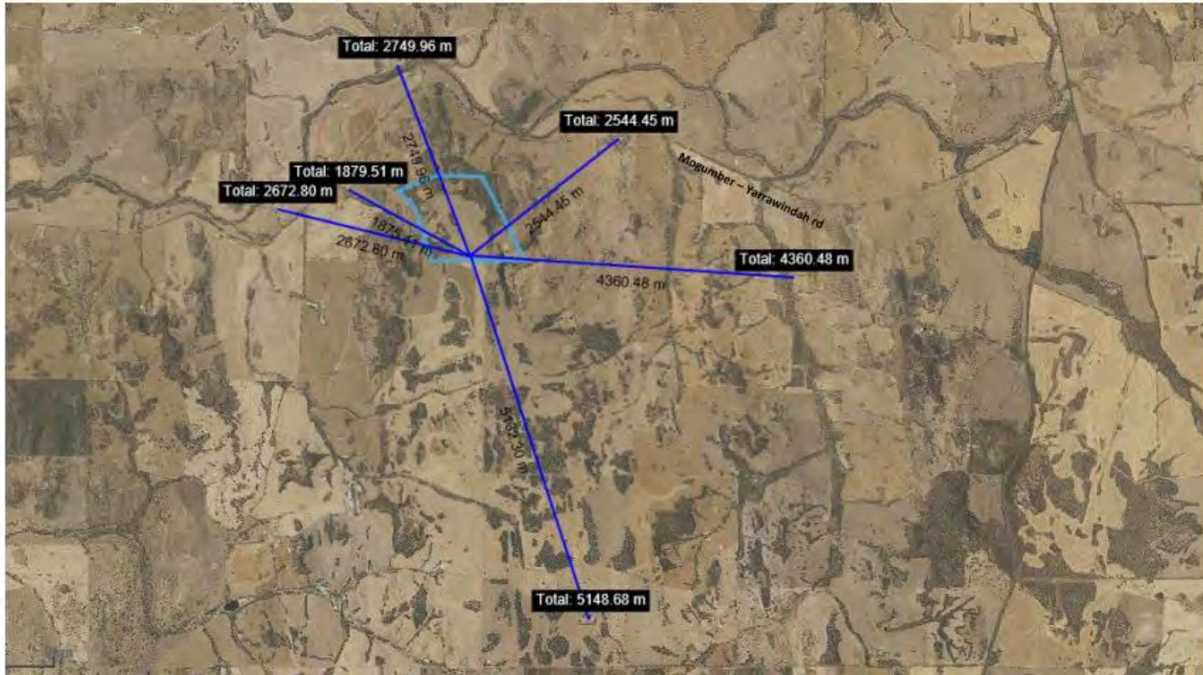
Figure 1 – Separation Distances – Composting facility to sensitive receptors
