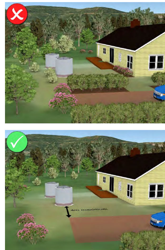
Figure 39: A good and bad example of landscaping around a water tank
