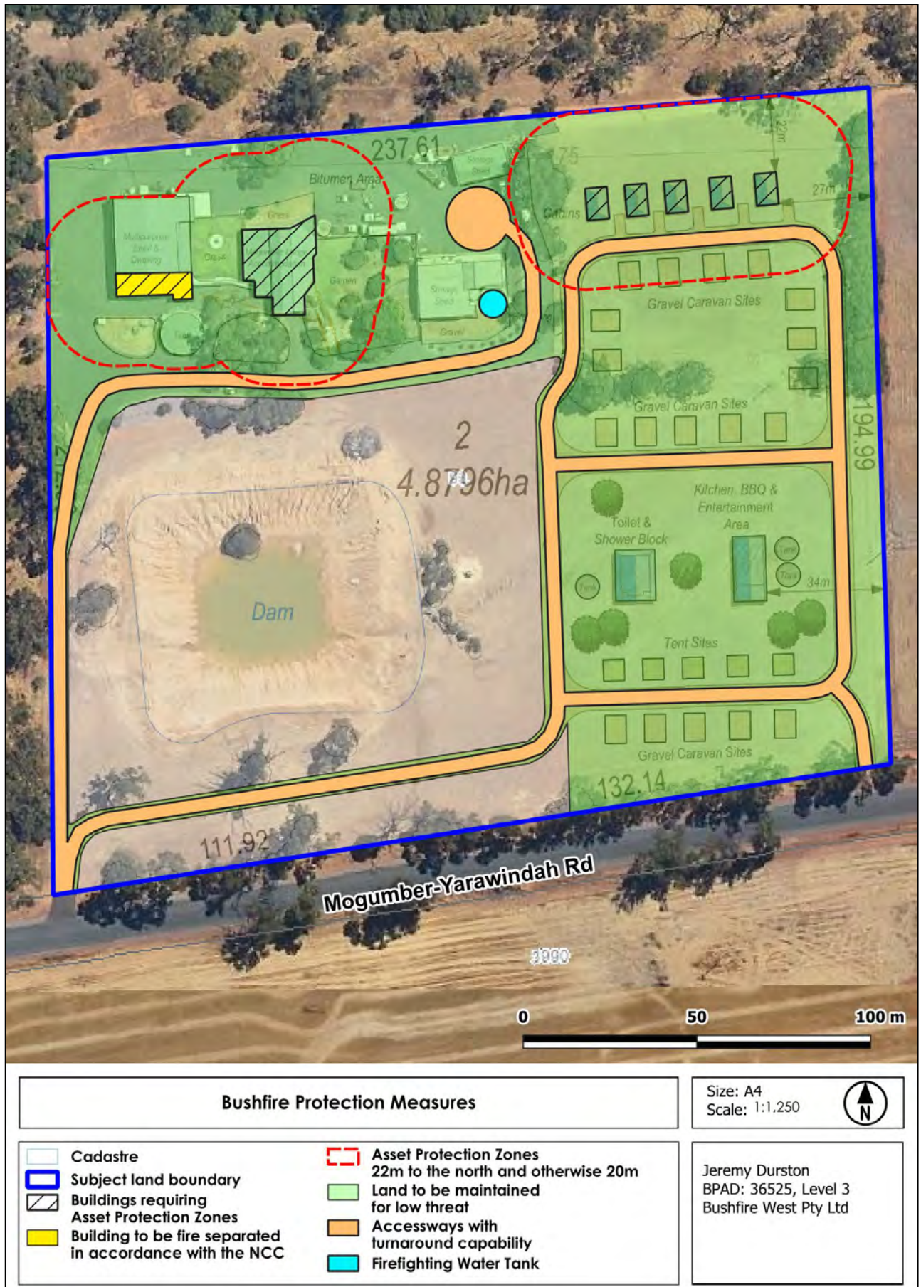
Figure 6: Bushfire Protection Measures
